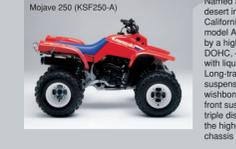
Named after the rugged desert in Southern California, this sport model ATV was powered by a high-performance, DOHC, 4-valve engine with liquid cooling. Long-travel swingarm front suspension, double wishbone independent rear suspension and triple disc brakes give it the highest performing chassis in its category.
